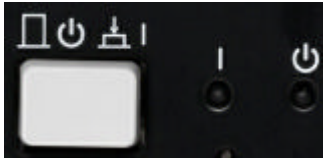
Fig. 2-4: Standby switch and LEDs
