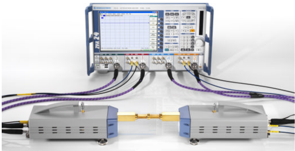
Fig. 2-6: Test setup for 2-port transmission measurement with R&S ZVA-Z110 (similar for the other models)
