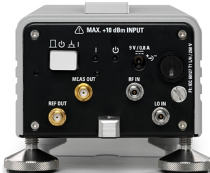
Fig. 2-3: Rear view of the frequency converter
